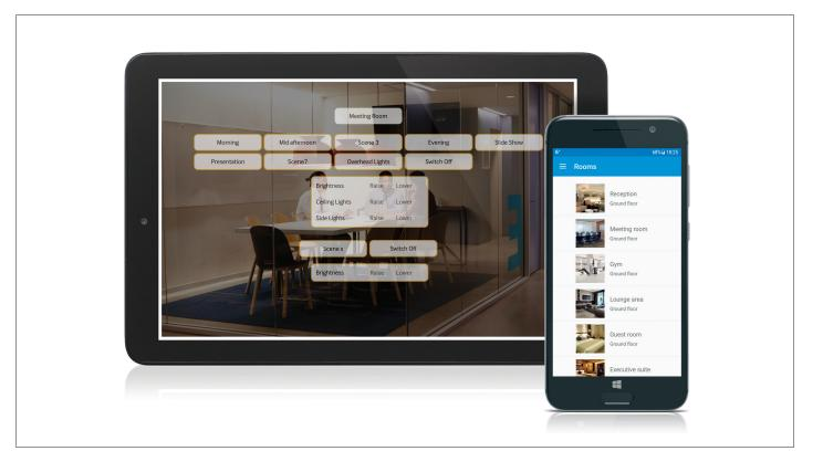
A touchscreen that allows the control of customised scene and switch control for a Rapid lighting control system. The look and feel of the scenes screens and the manner it controls the lighting zones is versatile and configurable exact to the needs of the project. Together with the flexibility and power capabilities of the Rapid lighting control system, every single light fixture can be switched and dimmed and controlled as part of the full system energy and comfort control regime.
